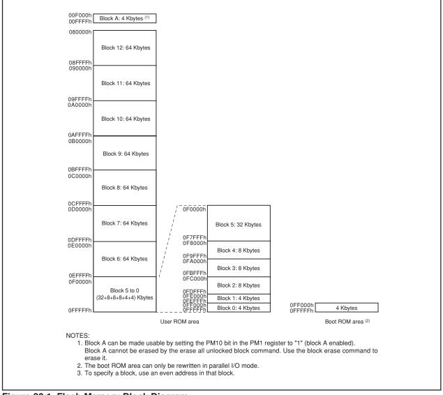
Figure 20.1 Flash Memory Block Diagram
